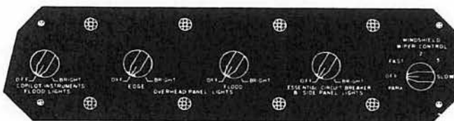
3 COPILOT'S AUXILIARY CONTROL PANEL
