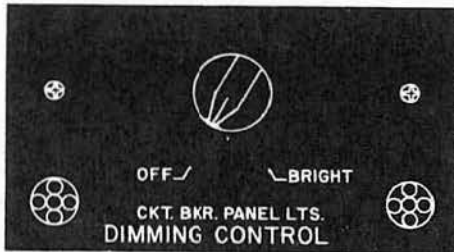
9 FLIGHT STATION DISTRIBUTION PANEL LIGHTS RHEOSTAT
